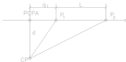
The slant distance  $d$  to the PCPA defines the data to be read from the Noise-Power-Distance(NPD)-curves; it defines also the elevation angle. The distance in the horizontal plane from the calculation point CP on the ground to the vertical projection of the PCPA defines the lateral distance for the calculation of the lateral attenuation (if relevant).
